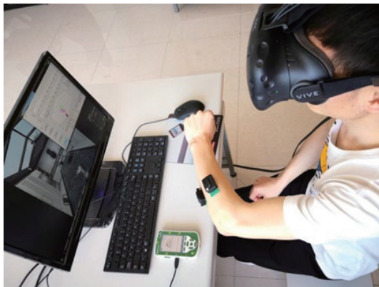
Fig.4 Real-time control with dual-channel sEMG
